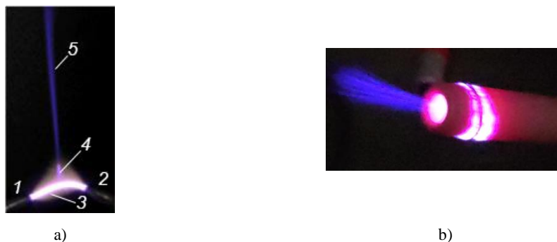
Fig. 1. (a) Apokampic discharge. 1, 2 – electrodes; 3 – discharge channel; 4 – bright branch; 5 – plasma plume. (b) Cold air plasma jet.
