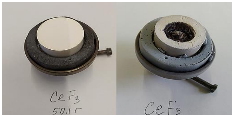
Fig. 1. the target from CeF 3 before (left) after evaporation (right).
